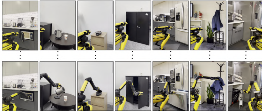
Fig. 1: Glimpse of some of the diverse robot manipulation capabilities across physical office and kitchen scenes enabled by our framework. We learn to predict point tracks from web videos for learning interaction plans that can be used for inferring robot actions in unseen scenarios. This enables a common goal-conditioned policy to perform everyday tasks like closing microwaves, pulling out drawers, flipping open toasters, pouring from jars etc. Columns show first and last images of rollouts from our policy.
