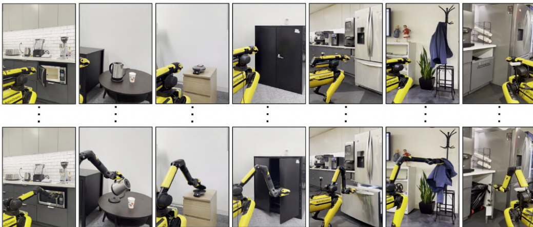
Figure 1: Glimpse of some of the diverse robot manipulation capabilities across physical office and kitchen scenes enabled by Track2Act . We learn to predict point tracks from web videos for learning interaction plans that can be used for inferring robot actions in unseen scenarios. This enables a common goal-conditioned policy to perform everyday tasks like closing microwaves, pulling out drawers, flipping open toasters, pouring from jars etc. Columns show first and last images of rollouts from our policy.
