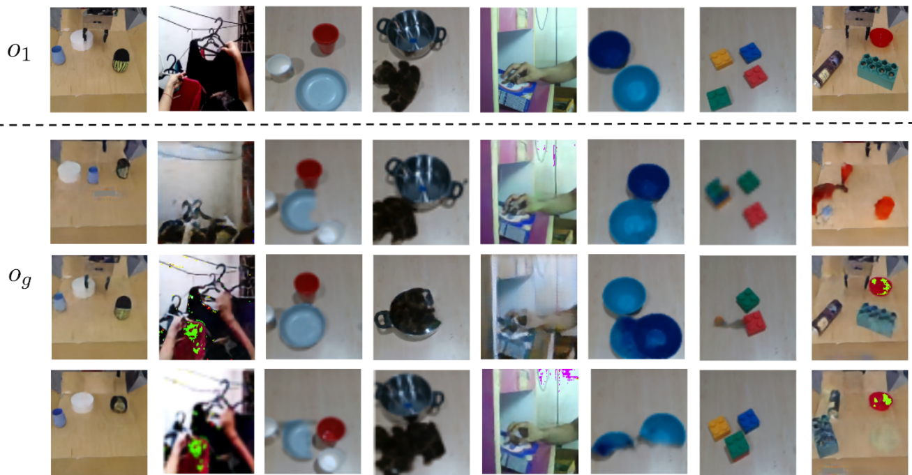
Fig. 7: Qualitative analysis of the affordance model, for random initial images. We choose o_1 to be a random unseen image, and show randomly sampled affordances o_g . We see that the sampled affordances o_g from our model are diverse and correspond to plausible interactions in the scene.
