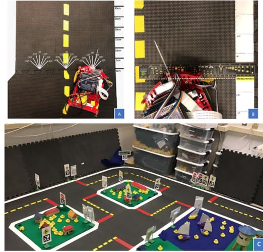
Fig. 2: **The Duckietown Environment:** (a) The initial pose setup for the Duckiebot in the real Duckietown environment. (b) A demonstration of distance measurement. (c) An overview of the Duckietown environment.
